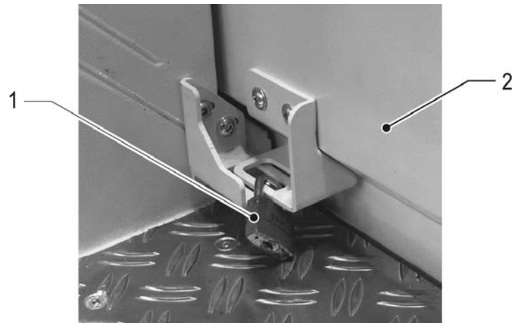
5.1.1.1 - 2 Work area safety door secured by padlock
